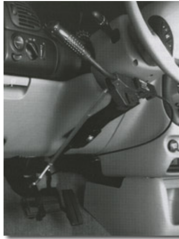
Figure 4.1: Mechanical hand control modification (Mobility Equipment-hand controls)
