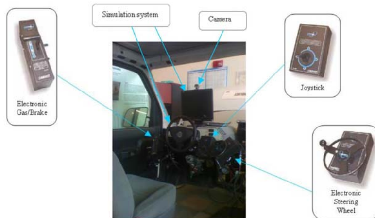
Figure 5.3: AEVIT DBW system connected to simulator system SSI
