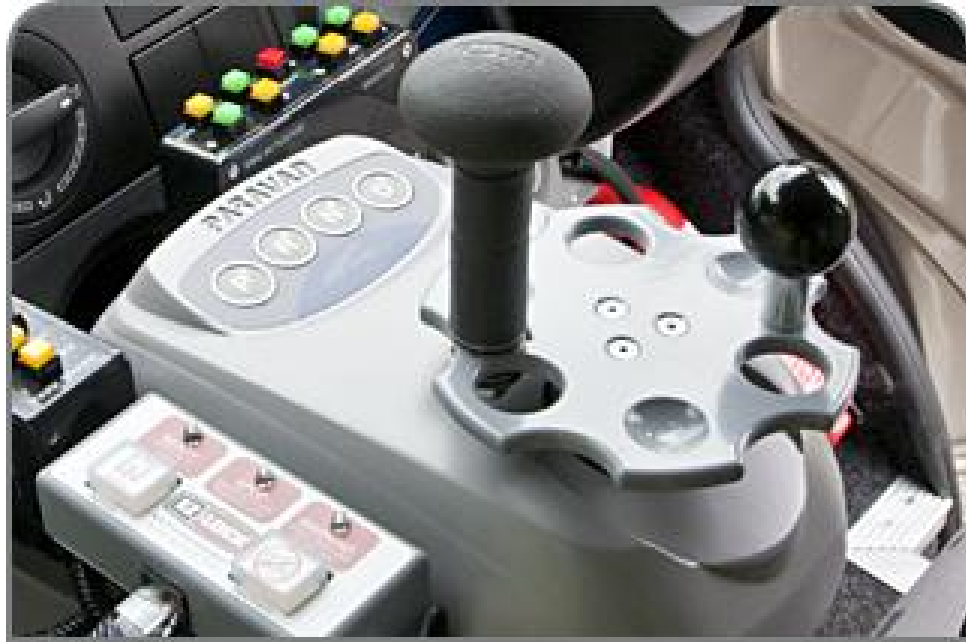
Figure 4.2: Reduced effort steering wheel (Space drive controls, 2009)
